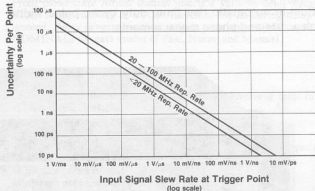
Graph 4, Trigger Level Timing Error: Affects the start and stop points of all time-interval measurements. Total error is the larger of the two trigger point errors.
